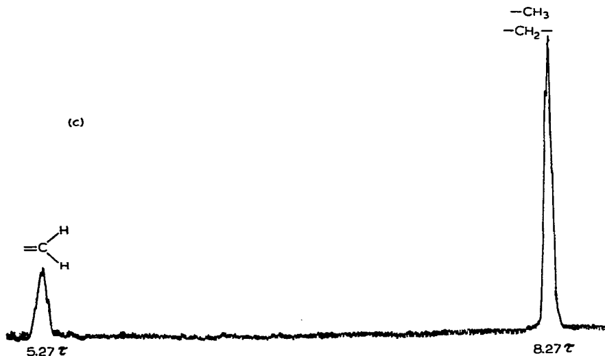
Fig. 1(c). 60 MHz spectrum at completion of reaction, showing the absence of ^{207}\text{Pb} - ^1\text{H} coupling.
